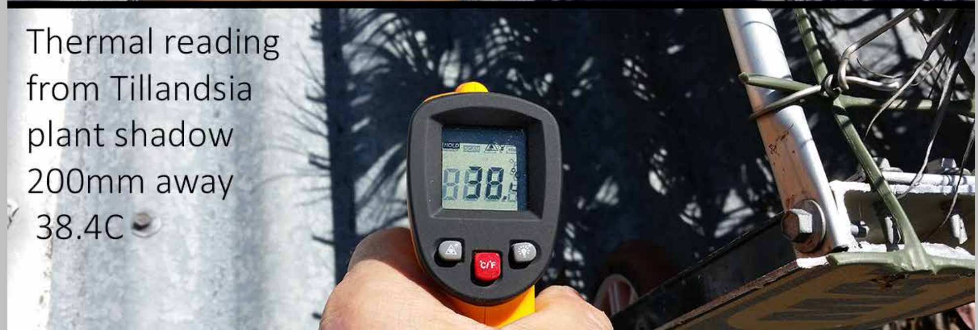
Temperature reading summer 2018 ambient air 30°C, iron roof 63.7°C shade from Tillandsias 38.4°C - heat mitigation on iron roof of 25.3°C
