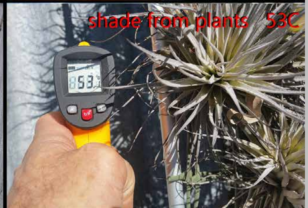
Temperature reading summer 2018 ambient air 42°C, iron roof 84.5°C, shade from Tillandsias 53.1°C - heat mitigation on iron roof of 31.4°C
