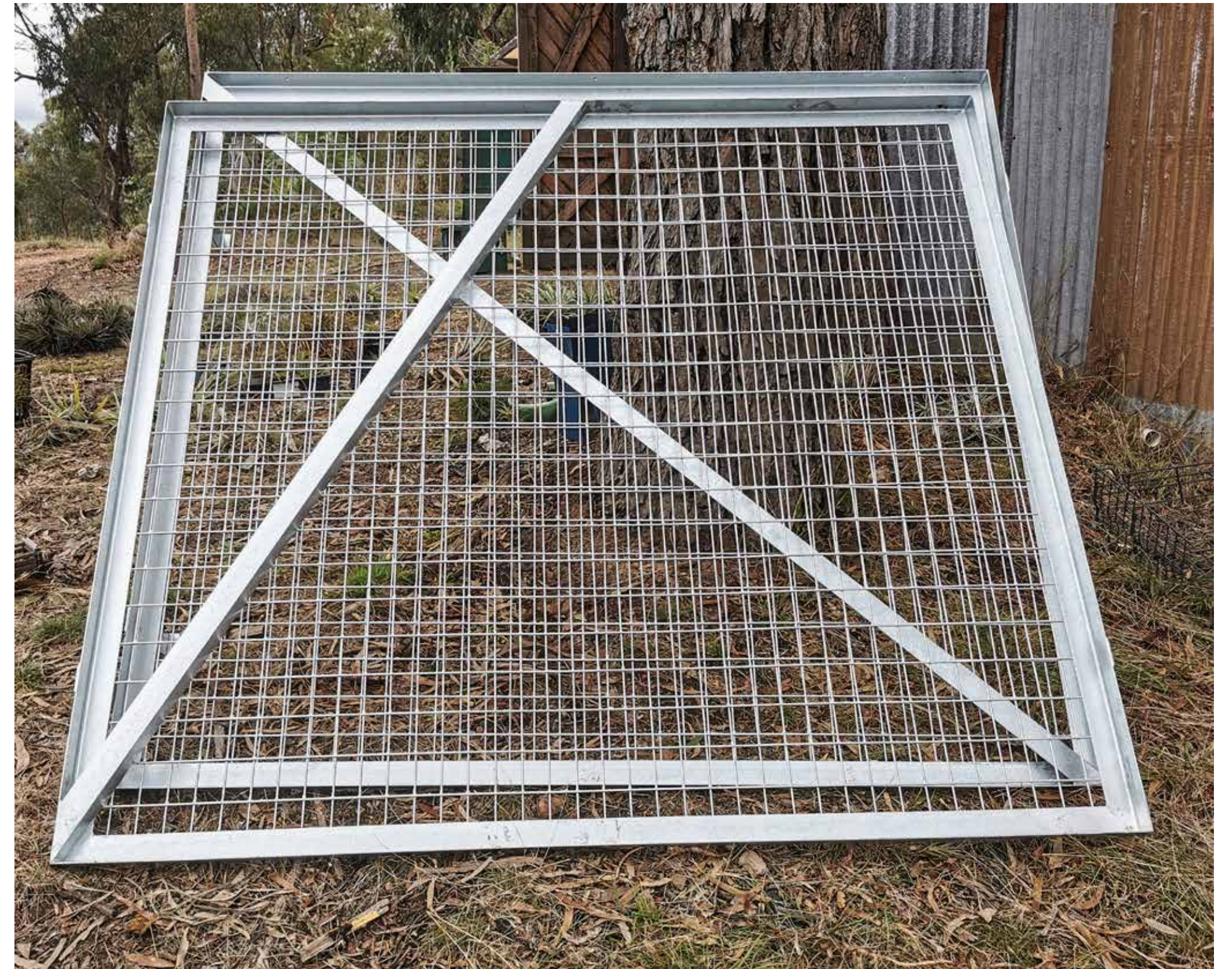
First two screen delivered ready for the installations of Tillandsias - the screens weigh in at 35 kg each.
