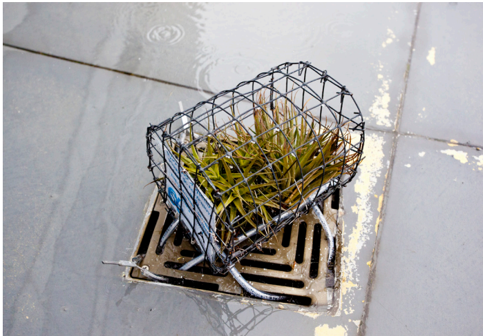
Tillandsia experimental test Cage anchored to a drain outlet.
