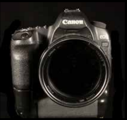
Canon EOS 5D Mark II - 21.1 effective megapixel full-frame CMOS digital single-lens reflex camera
